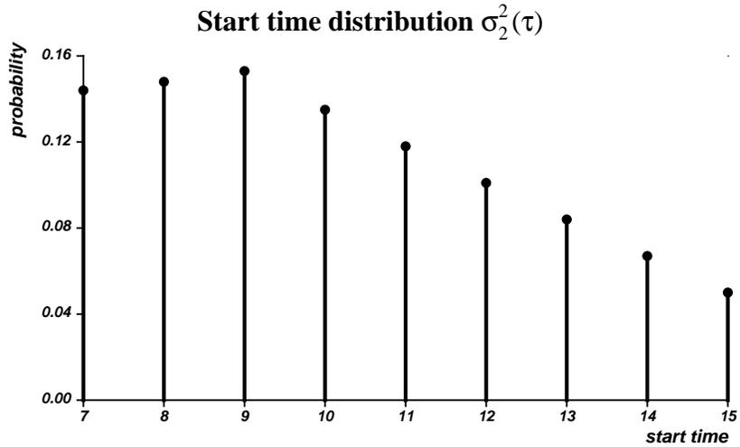
**Figure 3:** Start time distribution  $\sigma_2^2(\tau)$  for operation  $O_2^2$  in the initial search state for the problem defined in Figure 1.
